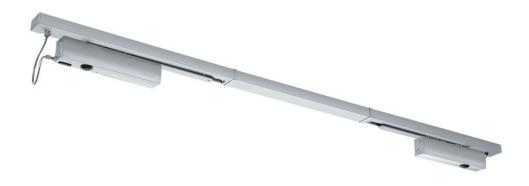
Overhead door closer system with guide rail on opposite hinge side for double leaf doors with anti-panic function up to 2800 mm hinge clearance with GEZE CB flex carry bar, integrated closing sequence control and electric hold-open device
