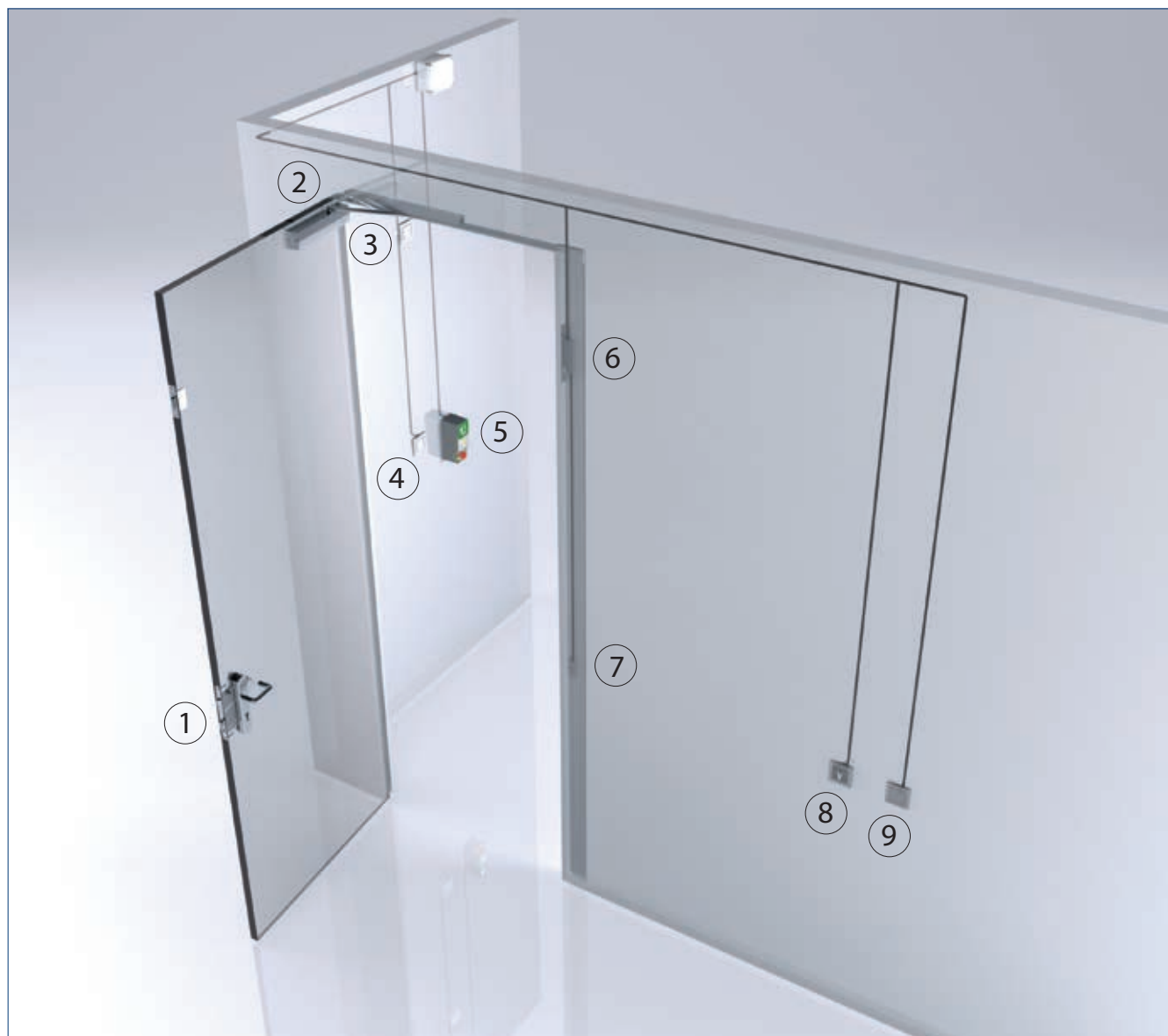
1 = panic lock with transmission function "E" on site | 2 = TS 4000/TS 5000 door closer | 3 = push button at 1.80 m height | 4 = switch to activate or deactivate the exterior push button | 5 = TZ 320 SN door control unit, surface-mounted/flush-mounted | 6 = FTV 320 escape door lock | 7 = A5000--B electric strike | 8 = key switch | 9 = push button outside
